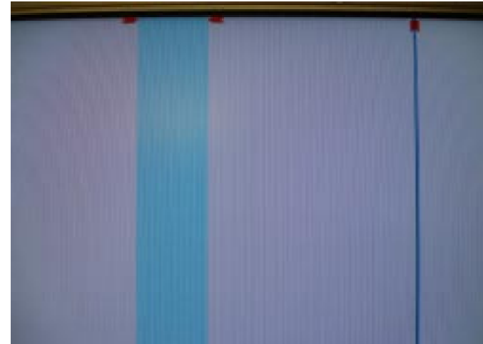
MULTIPLE TAB BOND FAILURE
