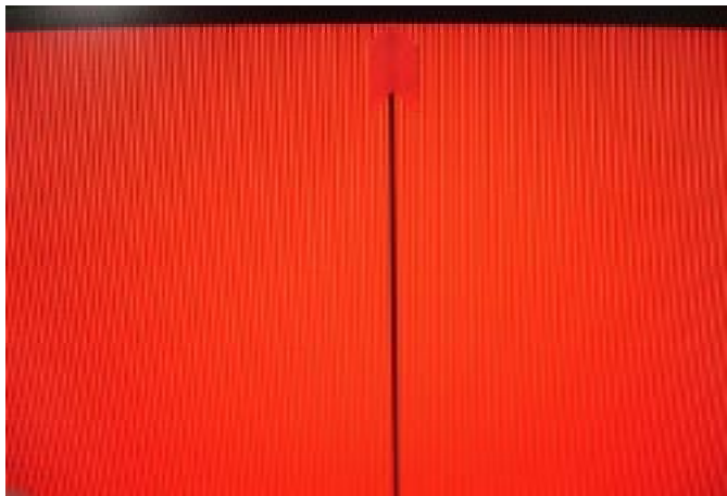
UPPER TAB BOND FAILURE
