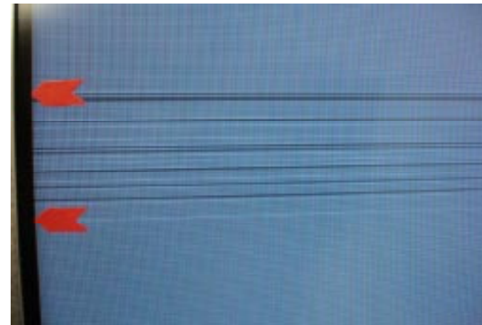
SIDE TAB BOND FAILURE
