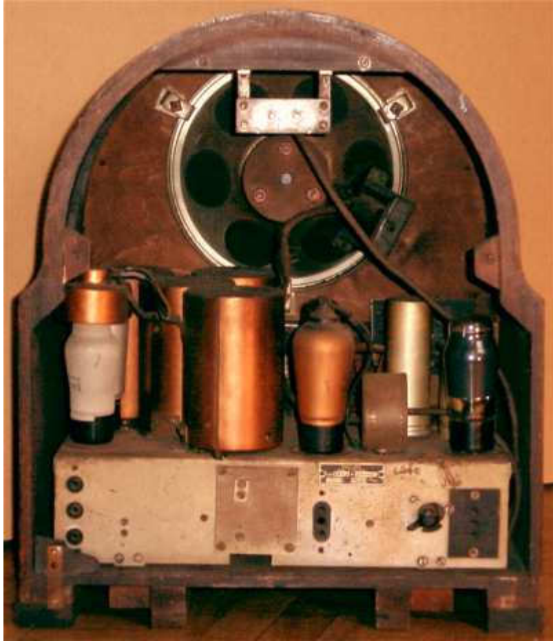
Rear view, dominated by the huge copper cans that conceal the "super" inductors.
