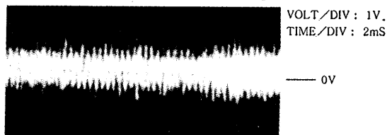
high tracking gain (higher fundamental wave than for low gain)
